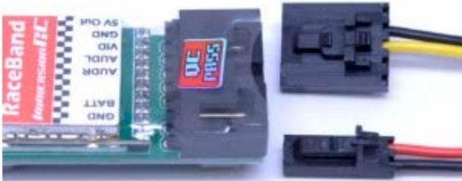
As you can see the camera power is not even represented on this image due to the fact that it is separately handled on your own installation. On the 5 pin Molex connector the only two signal lines required are the Video out from your camera (**YELLOW**) and the ground (**BLACK**). On the two pin connector the **RED** is connected to your battery positive lead and the **BLACK** is connected to your battery ground.
